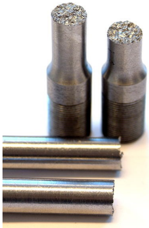
Cast Iron tensile test
