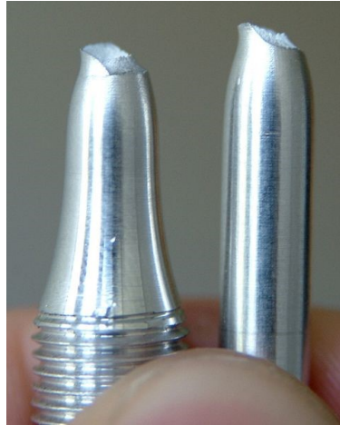
Aluminum tensile test
